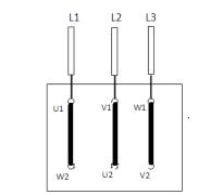
When Three Phase power supply of the above mentioned L1, L2, and L3 is given to U1, V1 and W1 terminals, it functions as -
