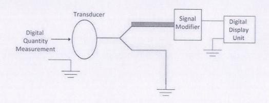
Data acquisition is the process of sampling signals that measure real-world physical conditions and converting the resulting samples into digital numeric values that can be manipulated by a computer.
