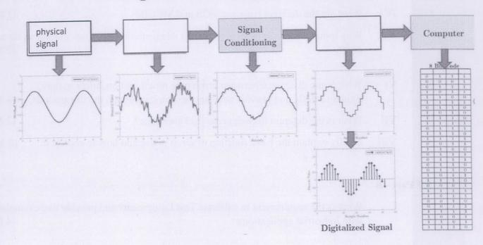
V Briefly explain the process of above block diagram according to the digital instrumentation application. What do you think the given physical signal and digitalized signal as well as computer? (4 Marks)
