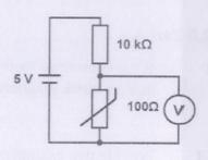
II. In the example above a 10K resistor (R1) is connected in series with a thermistor (R2) to create a voltage divider. The total voltage across both components is 5.0V. When the thermistor is placed in a warm environment it has a resistance of  $100\Omega$ . Calculate the voltage across the thermistor under these conditions.
